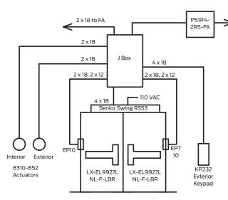
Operation: KP232 keypad exterior to signal EL latch retraction and enable exterior actuator through LX switches in panic device. Interior actuator always active.
