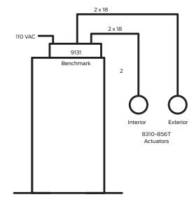
Operation: No latching at this door. For a single occupancy restroom. Either actuator will open door at any time.
